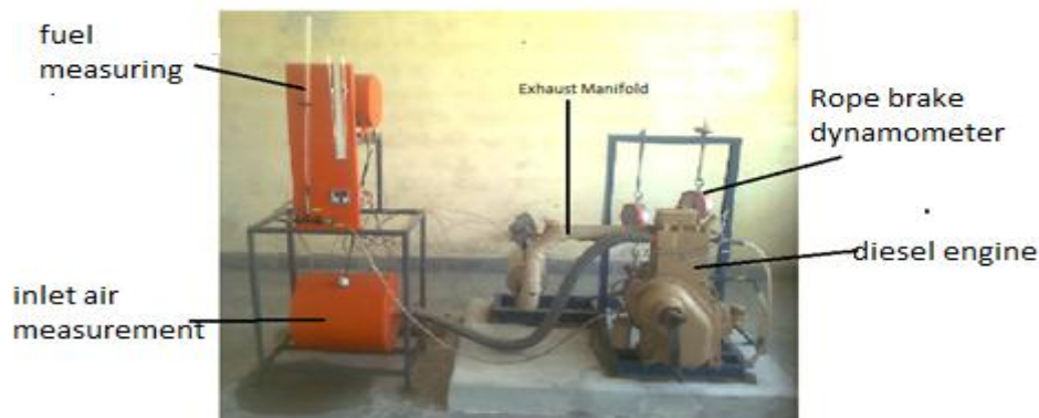
Figure 2 Pictorial diagram of experimental setup
