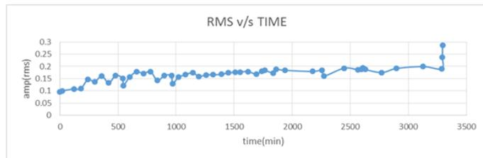
Fig 2(b) rms v/s time graph at 3000 rpm & 400 psi load
