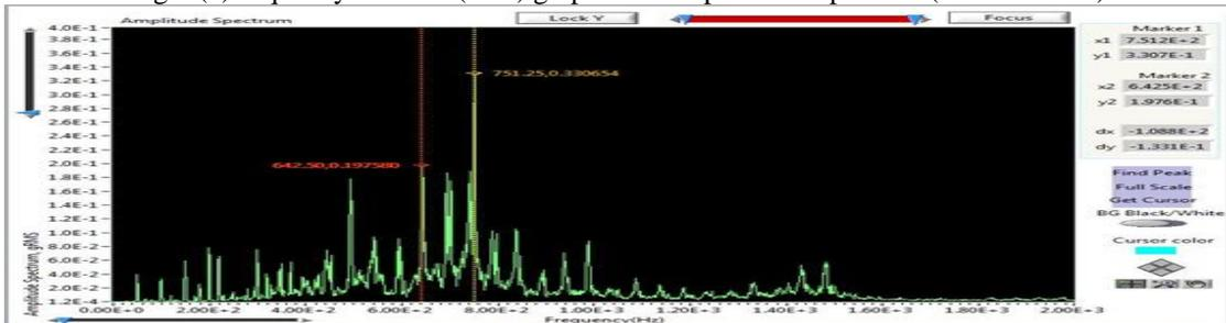
Fig 6(a) frequency v/s time (FFT) graph at 3000rpm & 400 psi load (at start)
