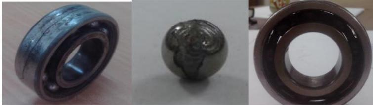
Fig 11(a) Defect at 300 psi (O R fault) (burning)
