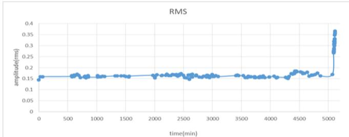
Fig 2(a) rms v/s time graph at 3000 rpm & 300 psi load
