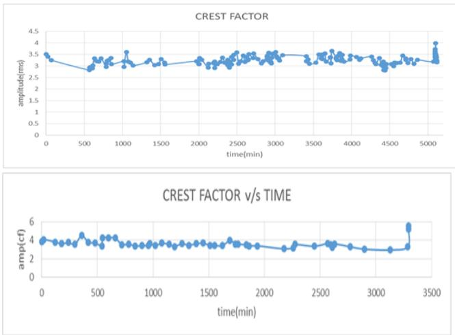
Fig 4(a) crest factor v/s time graph at 3000 rpm & 300 psi load
