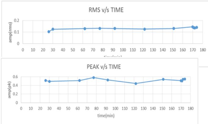
Fig 2(c) rms v/s time graph at 3000 rpm & 500 psi load
