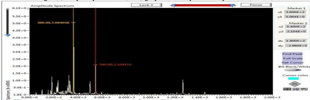
Fig 8 (b) frequency v/s time (FFT) graph at 3000rpm & 300 psi load (before failure)
