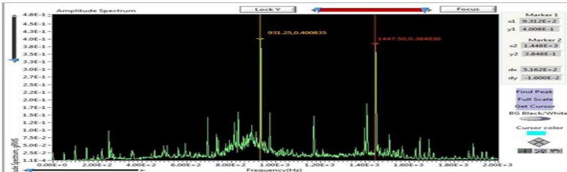
Fig 7(a) frequency v/s time (FFT) graph at 3000rpm & 500 psi load (at start)
