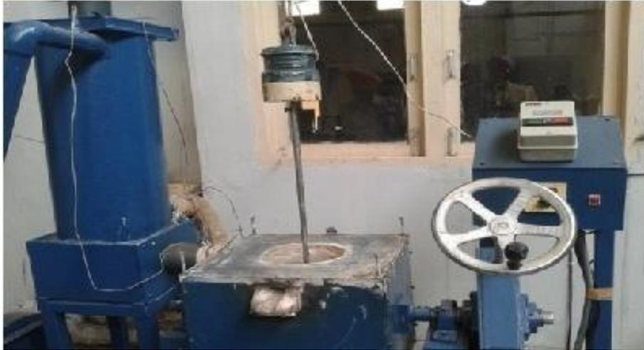
**Figure 1:** Oil fired muffle furnace used for fabrication of MMC and hybrid MMC
