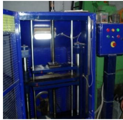
Figure 7(b): Fatigue test rig
