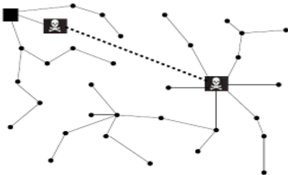
Fig. 2.4 A laptop-class adversary using a wormhole to create a sinkhole in TinyOS beaconing.
