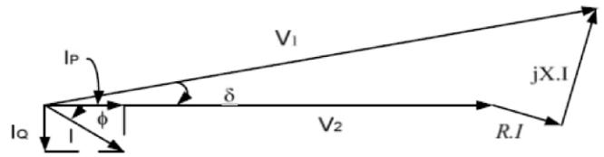
Fig-2 Phasor diagram without compensation
