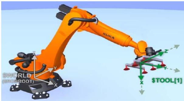
FIG.9: TOOL COORDINATE SYSTEM
