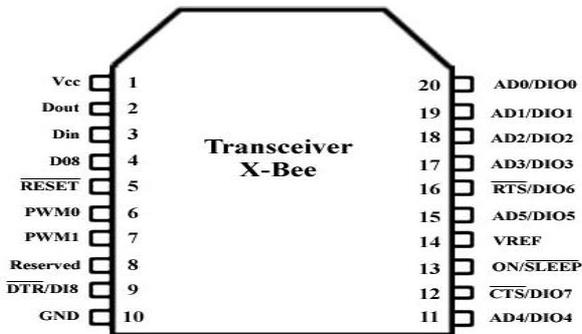
Figure 6. Pin Diagram of Zigbee Transceiver
