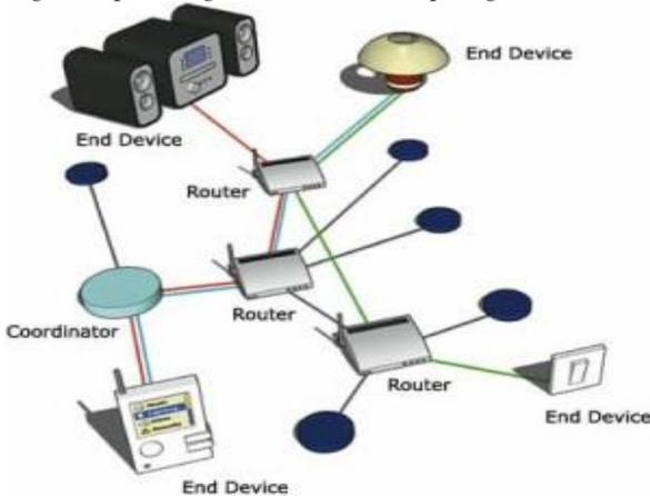
Figure-1 Zigbee Communication Operation
