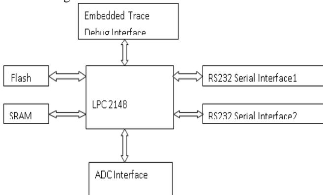
Figure 3.The Hardware Structure of Processing Terminal.
