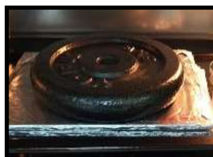
Fig. 2: Drying process of chitin cake in the oven at 120 °C
