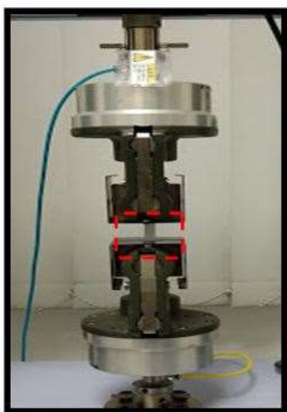
Fig. 3: Testing the mechanical strength of chitin strip
