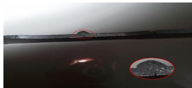
Fig.5. Plain tensile test specimen - Fails at base metal
