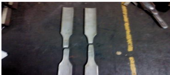
Fig.7. Tensile test specimen (GTAW)
