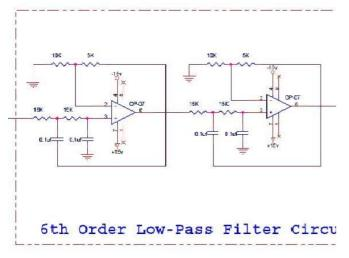
Butterworth filters are termed maximally - flat-magnituderesponse filters, optimized for gain flatness in the pass-band. The attenuation is -3 dB at the cutoff frequency . Above the cutoff frequency the attenuation is -20 dB/decade/order. The transient response of a Butterworth filter to a pulse input shows moderate overshoot and ringing.[10]
