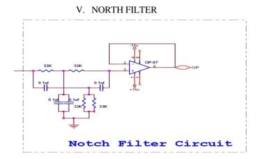
A band reject (band stop) filter is a filter passes the most part of frequencies unchanged but attenuates other frequencies to very low levels in a certain range. [4] A notch filter actually can also be perceived as a band stop filter with a high Q factor, i.e. it often wants to filter out the undesired signal in the specific frequency (e.g. noise) only . However, the conventional band stop filter usually has a relatively wide stop band [2]
