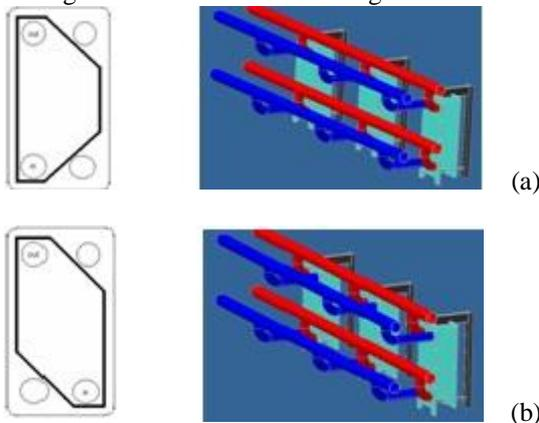
Fig. 7 (a) Parallel Flow Arrangement
