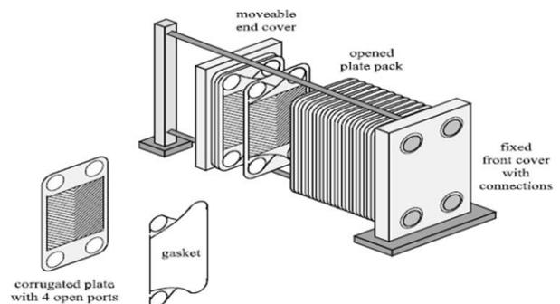
Fig. 1 Assembly of PHE
