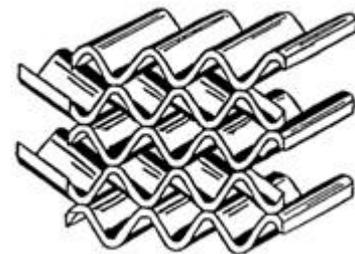
Fig. 4 Corrugations on Heat Transfer Plate
