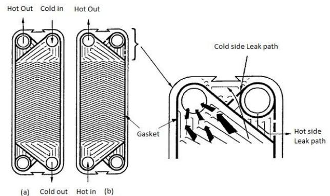
Fig. 2 Typical Heat Transfer Plate
