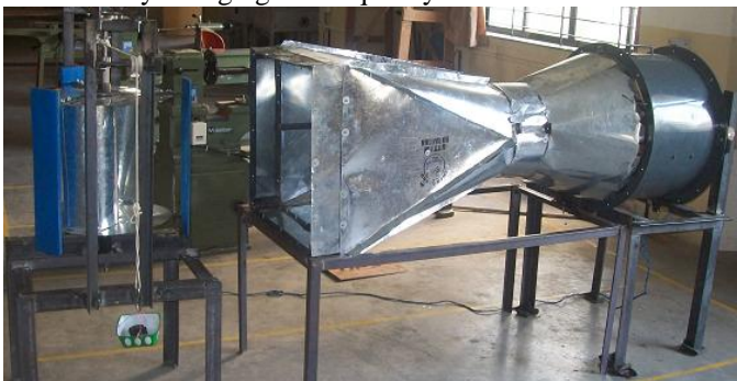
Fig.3 Test Set-Up Savonius middle of H-rotor in Wind Tunnel
