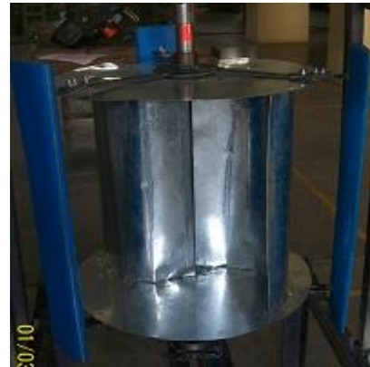
Fig.2 Combined Savonius-H-darrieus Rotor.
