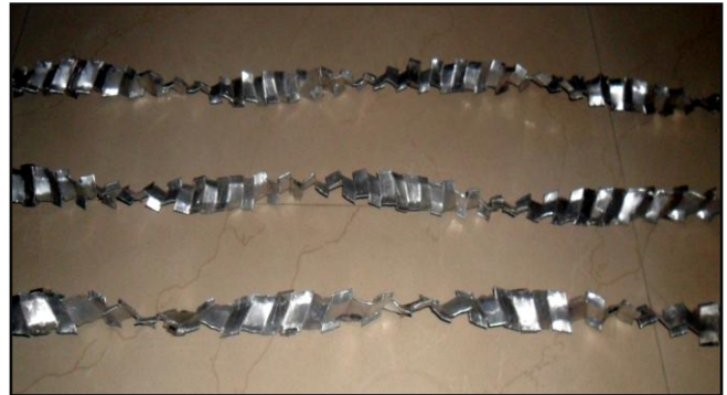
Fig. 3. Actual view of cut corrugated twisted tape insert
