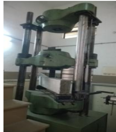
Fig. (3) UTM for flexure strength testing
