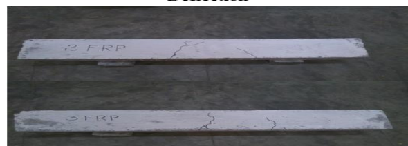
Figure 7: Crack patterns in 50% and 75% GFRP reinforcement
