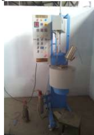
Fig.2. Stir casting setup
