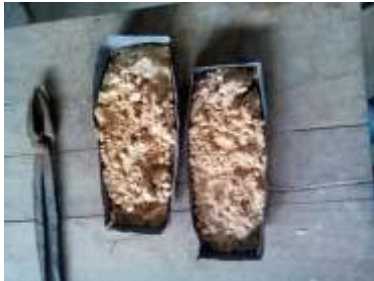
Fig 1. Groundnut shell ash (GSA) after carbonization
