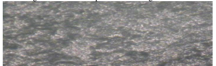
Fig 3.1.4b Al+6% Grp after sintering at 20x
