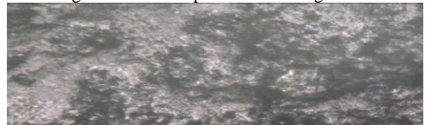
Fig 3.1.6b Pure Grp after sintering at 20x
