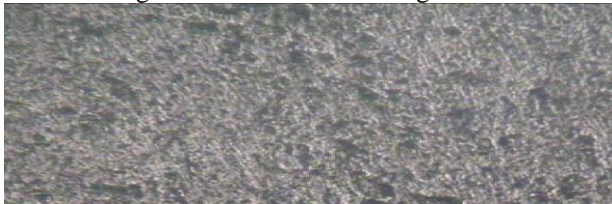
Fig 3.1.1a Al after sintering at 20x
