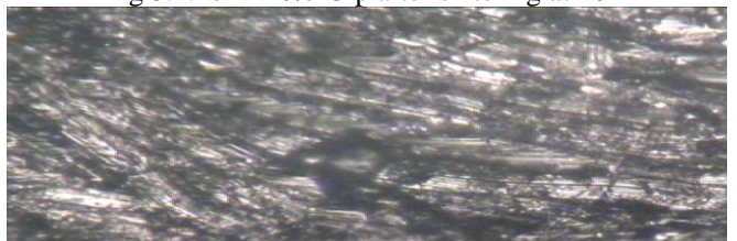
Fig 3.1.5a Al+8% Grp before sintering at 20x
