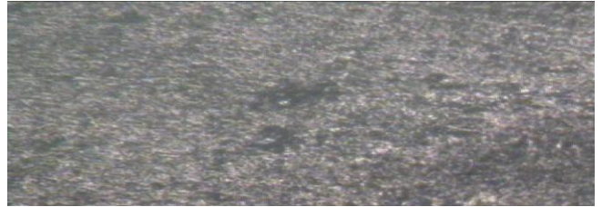
Fig 3.1.3b Al+3% Grp after sintering at 20x
