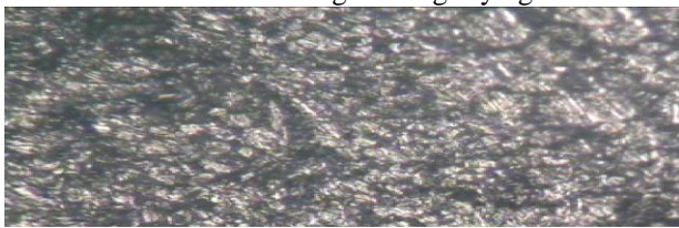
Fig 3.1.1a Al before sintering at 20x
