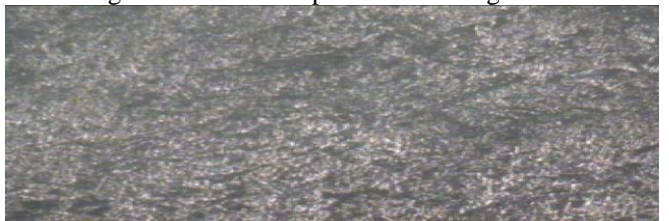
Fig 3.1.5b Al+8% Grp after sintering at 20x
