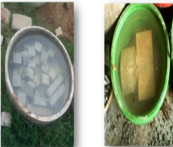
Fig. 4 1) curing in normal water 2) Curing of cubes in HCL Solution
