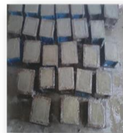
Fig. 3 casting of cubes
