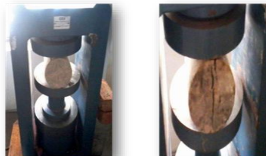
Fig. 6. Testing of cylinders
