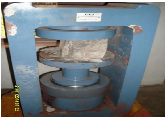
Fig 5: Testing of Cubes
