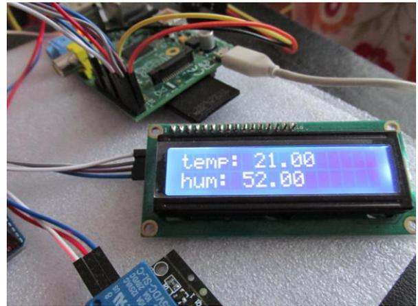
Fig. 5: Temperature and Humidity values on LCD
