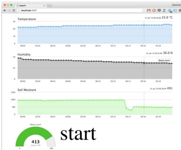
Fig.7: Web interface of the 'Remote plant watering and monitoring system based on IoT'
