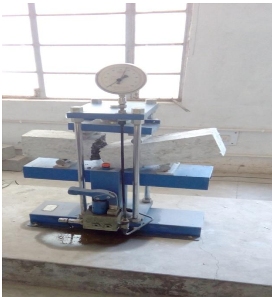
Fig.4 Test set up for Flexure Strength
