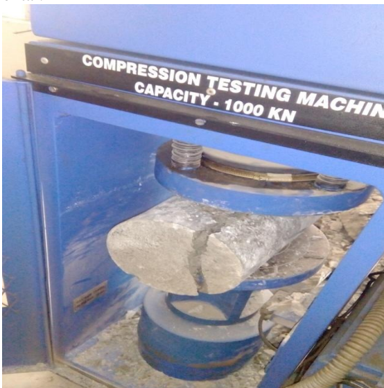
Fig.5 Test set up for Split Tensile Strength
