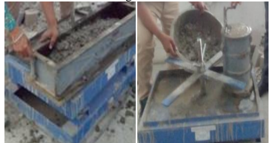
Fig.2 Casting of cubes, beams and cylinders
