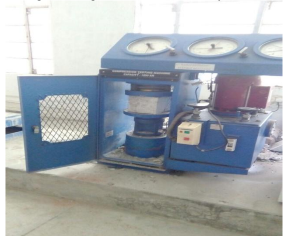
Fig.3 Test set up for Compressive Strength
