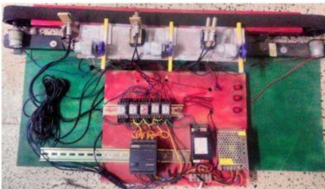
Above Fig. clearly shows that working of objects sorting system. A belt conveyor is used to feed the iron objects. It is driven by means of a the proximity sensors are use to sort the iron objects when actuated by the sensors. further the DC motor get activated and push the valve forward which push the iron object and sort the by height. Object such as boxes, packing load onto the conveyer belt. We are using for auto loader mechanism, then the different sizes objects moving toward the conveyer
