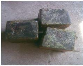
Test Specimens of High Strength SCC mix of M100 grade immersed in HCL solution
