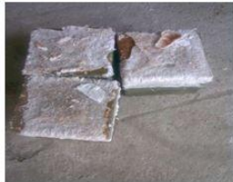
Test Specimens of High Strength SCC mix of M100 grade immersed in Na2SO4 solution
