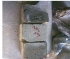
Test Specimens of High Strength SCC mix of M100 grade immersed in Na2SO4 solution
