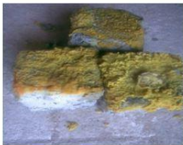
Test Specimens of High Strength SCC mix of M100 grade immersed in H2SO4 solution
