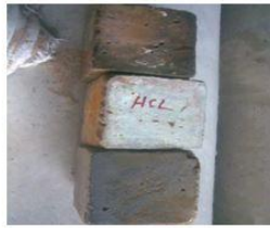
Test Specimens of High Strength SCC mix of M100 grade immersed in HCL solution
