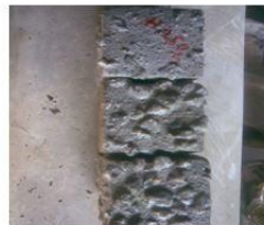
Test Specimens of High Strength SCC mix of M100 grade immersed in H2SO4 solution
