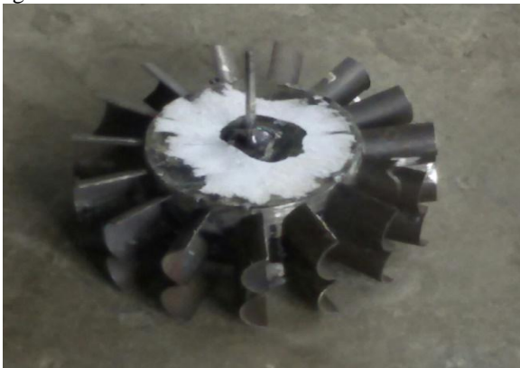
Fig-7 Pelton Wheel Turbine
