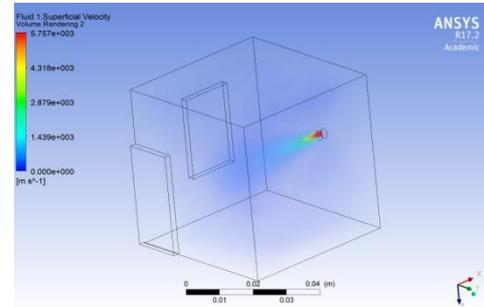
Fig. 17. The flow of air from cooler outlet to room of size 10ft x 10ft
