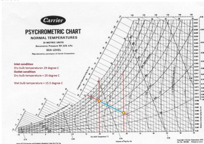
Fig. 1. Air cooling process; Psychrometry chart source-
