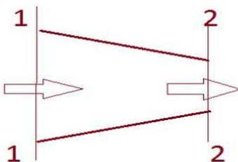
Fig. 13. Nozzle effect due to shape of cooler
