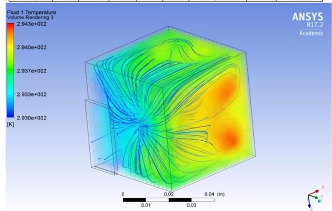
Fig. 18. Cooler outlet air and fresh air flow analysis
