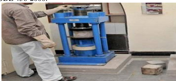
Compressive test machine
