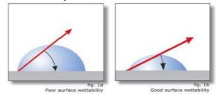
Above figure illustrate the difference between good and poor wettability. The higher the surface energy of the solid substrate in relation to the surface tensions of the liquid, the better its wettability, and the smaller the contact angle. In order for a proper bond to exist between a liquid and a substrate surface, the substrate's surface energy should exceed the liquid's tension by about 2-10 mN/m.
