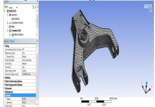
Fig.6.Meshing of Upper Control Arm using Tetrahedral Element
