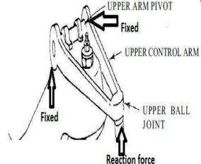
Fig.2. Boundary forces for Static Condition *B. Condition II: Static and Dynamic loads*
