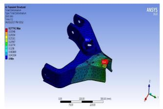
Fig.8. Deformation of Upper Control Arm The maximum deformation 0.37741mm and von mises stress is 146.14 MPa obtained.
