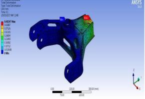
Fig.13. Deformation of Upper Control Arm
