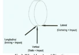
Fig.3. Wheel Loads and Directions
