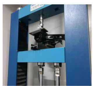
Fig.14. Testing of Arm on UTM
