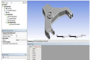
Fig.9. Natural Frequency of Upper Control Arm *B. Modal Analysis:*
