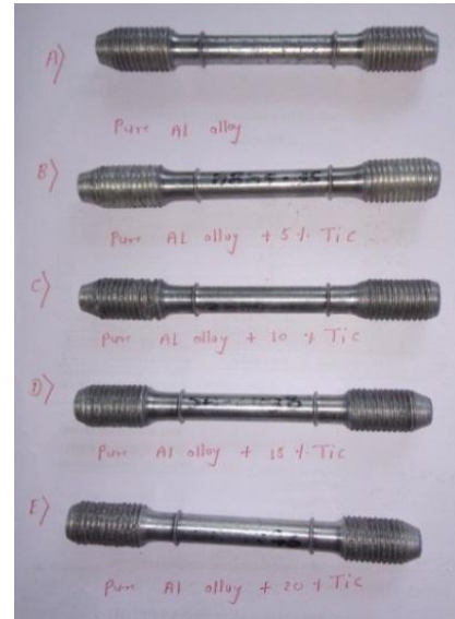
Fig.3 Photograph of tensile test specimens for various wt % of TiC particles of LM28/TiC composites.
