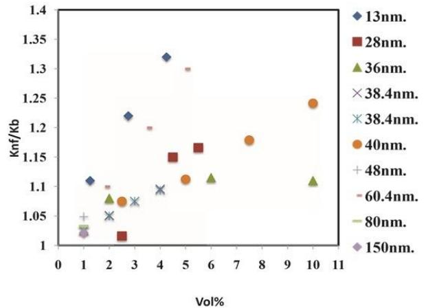
Figure 2. Effect of particle size on thermal conductivity of nanofluid.
