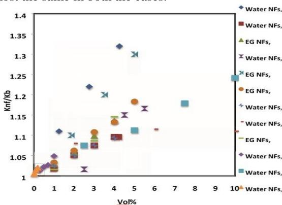
Figure 1. Effect of volume fraction of nanoparticles on ratio thermal conductivity of  $Al_2O_3$ -based nanofluids
