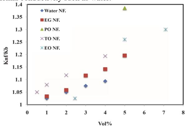
Figure 3. Effect of base fluid on thermal conductivity of nanofluid.
