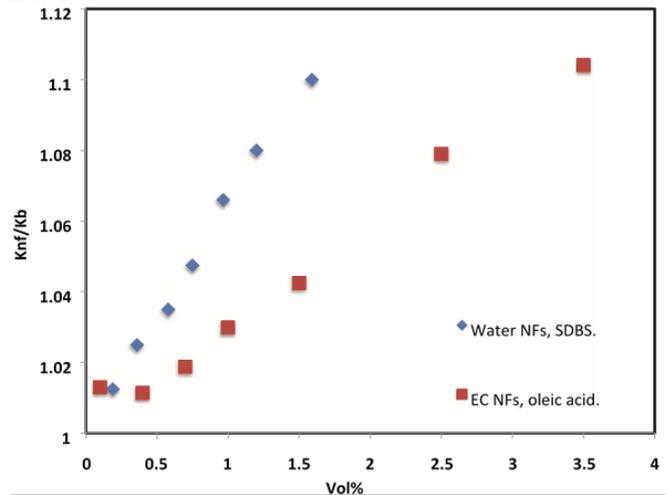
Figure 8. Effect of additives on thermal conductivity of nanofluid.
