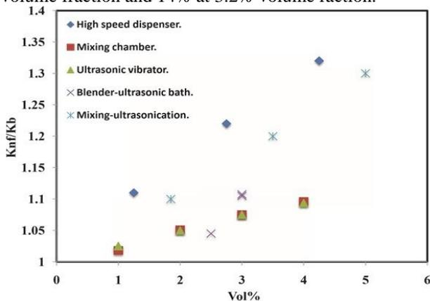
Figure 4. Effect of preparation method on thermal conductivity of nanofluid.
