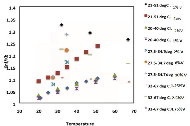
Figure 5. Effect of temperature on thermal conductivity nanofluid.
