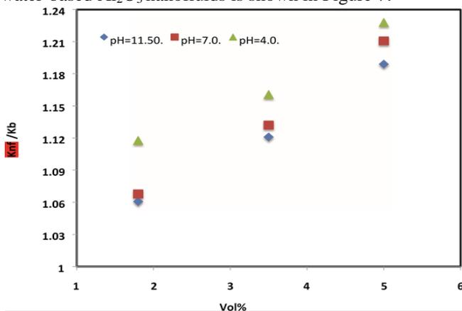
Figure 7. Effect of pH on thermal conductivity of nanofluid.
