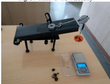
Fig. 6. Determination of coefficient of friction
