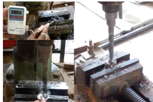
Fig. 11. Oil feed, Temperature measurement and drilling (to limit the quantity of oil). Only three spoons of the oil (12 ml) was poured during operation. The temperature of the 'MS job' was recorded (refer Fig.11).
