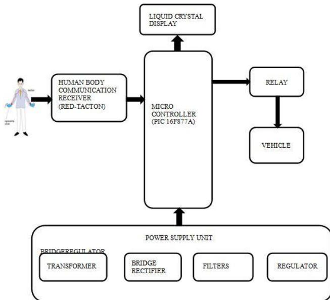
Fig.2. Receiver Side of Human Body Communication
