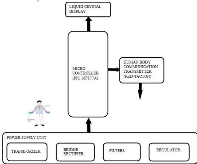
Fig.1. Transmitter side of Human body communication
