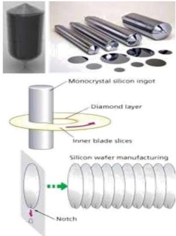
Fig: 3 Ingots and Wafer Preparation
