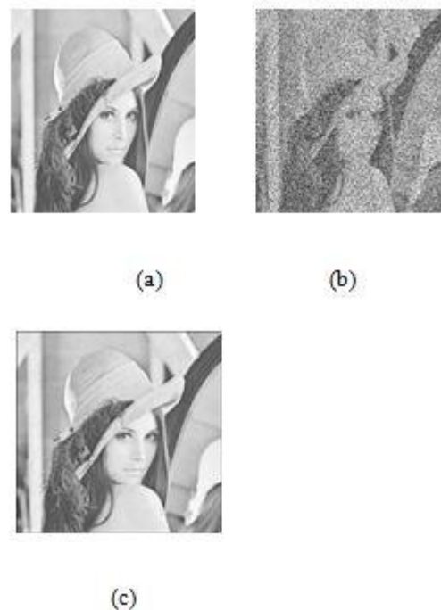
Fig: (a) Lenna original image (b) Noisy image(50% noise added) (c) Restored image(PSNR=29.0388 db)
