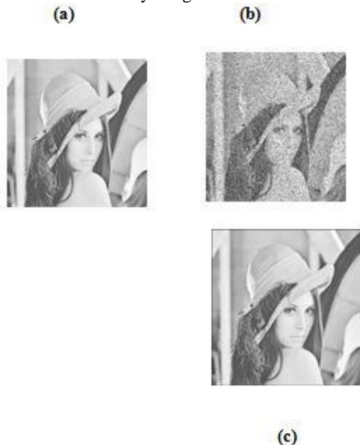
Fig: (a) Lenna original image (b) Noisy image(30% noise added) (c) Restored image(PSNR=33.0972 db)
