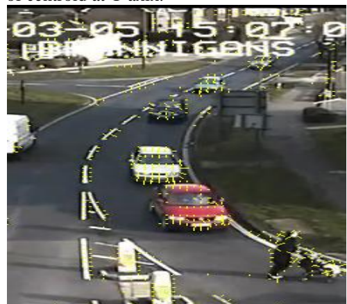
Figure 4: Key point of object using SURF or key descriptor
