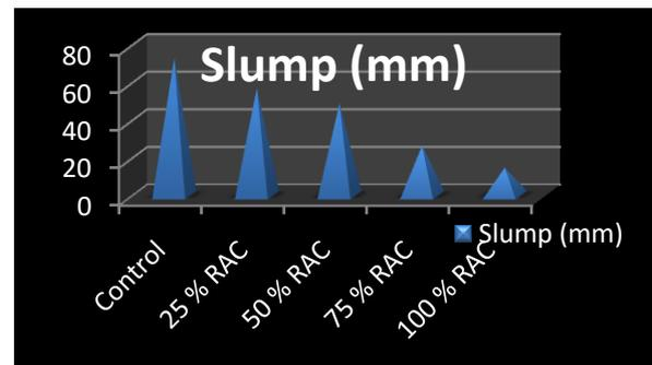
Fig 3.Slump variation of various mixes
