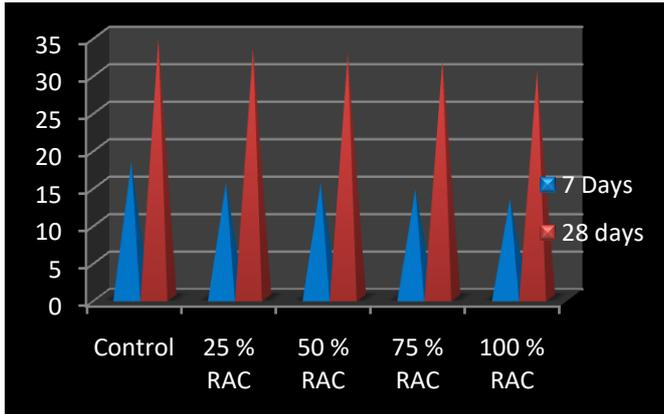
Fig4: Compressive strength of various mixes
