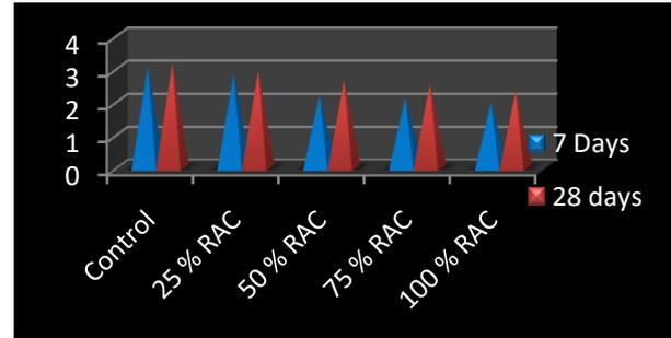
Fig 5: Split tensile strength of various mixes
