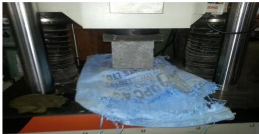
Fig 1 Compressive Strength Test Of Cube on UTM
