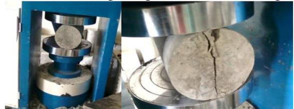
Fig 4: Loading arrangement for Split Tensile Strength Test.
