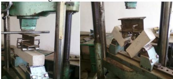
Fig 3: Flexure testing of beam.
