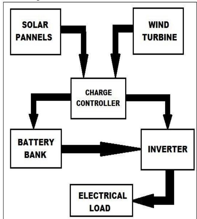
Figure 3. Block diagram of Hybrid energy generation system
