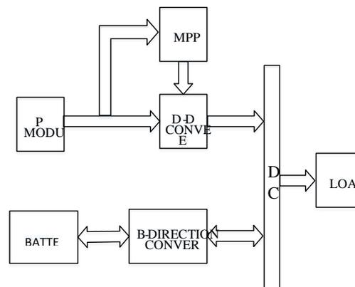
Figure. 1. Overall block diagram of PV energy system
