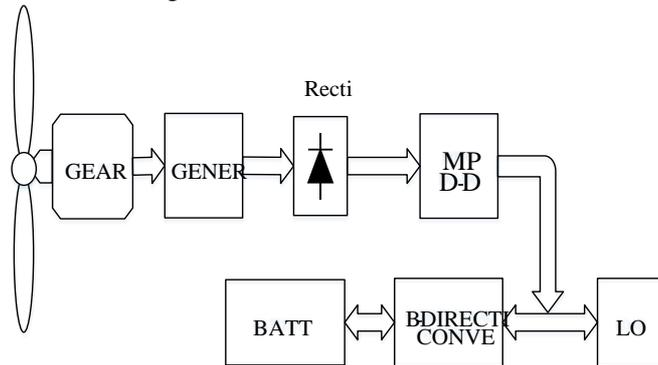
Figure. 2 Overall Block diagram of wind energy system
