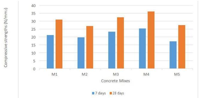
**VARIATION OF COMPRESSIVE STRENGTH OF FLY ASH AND SILICA FUME CONCRETE IN N/mm<sup>2</sup> FOR DIFFERENT MIX PROPORTIONS:**
