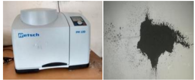
Fig 4: (a) PM 100 High energy ball mill (b) CuO nanopowder
