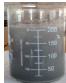
Fig 5: MgO-CuO nanofluid at 1%
