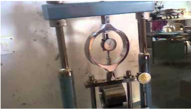
Fig 5: Marshall Stability testing of bituminous concrete specimen
