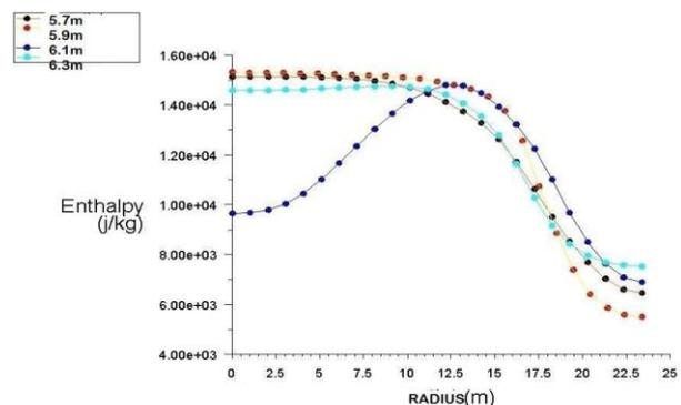
Figure 4 : Comparison between enthalpy and outlet radius at different air inlet height
