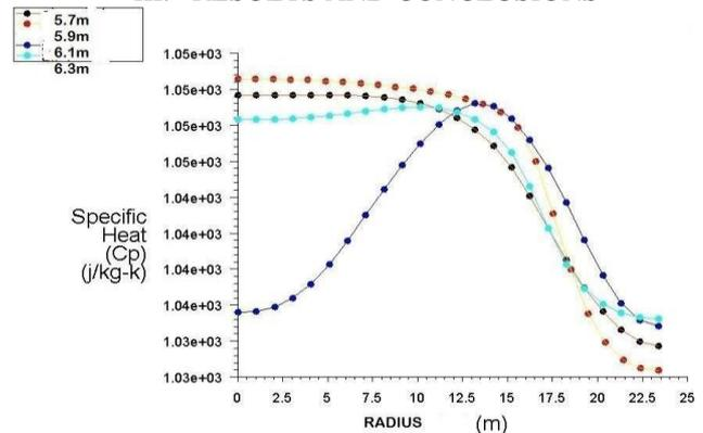
Figure 3 : Comparison between specific heat and outlet radius at different air inlet height
