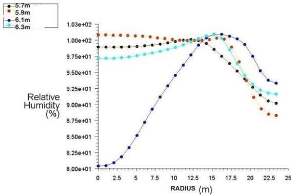
Figure 5: Comparison between relative humidity and outlet radius at different air inlet height
