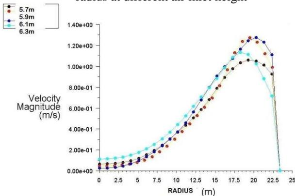
Figure 6: velocity and outlet radius at different air inlet height
