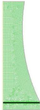
Figure 2: Meshed model of cooling tower.
