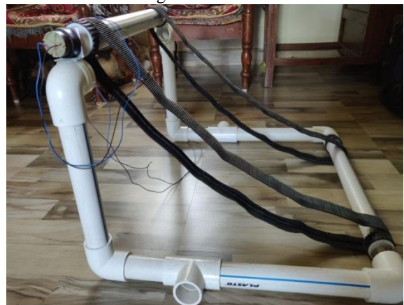
Fig: Fabrication of conveyer mechanism
