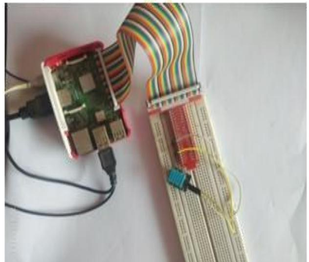
Figure 2: DHT11 Sensor with Raspberry Pi
