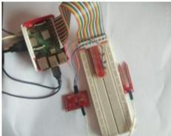
Figure 3: Soil Moisture Sensor with Raspberry Pi
