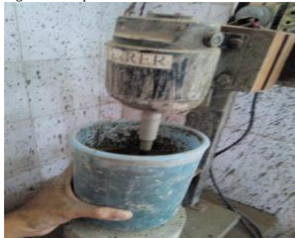
Fig. 1: Mixing Mechanism of raw grout material
