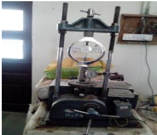
Fig. 12: Unconfined Compressive Strength test
