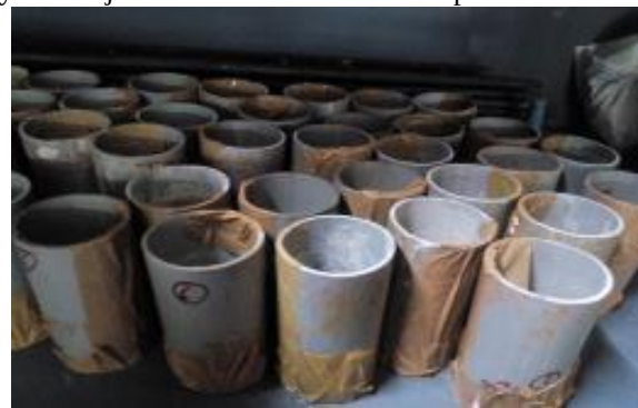
Fig. 11: PVC mould covered with cello tape for UCS specimen
