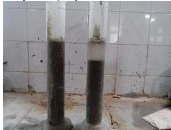
Fig. 5: Bleeding Potential test
