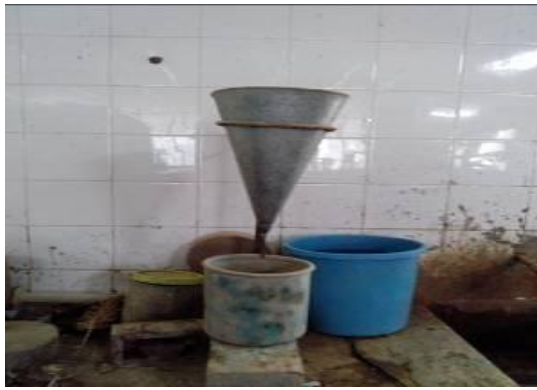
Fig. 2: Set up for Marsh Cone Test
