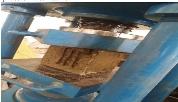
Figure II: Cube under Compression testing Machine
