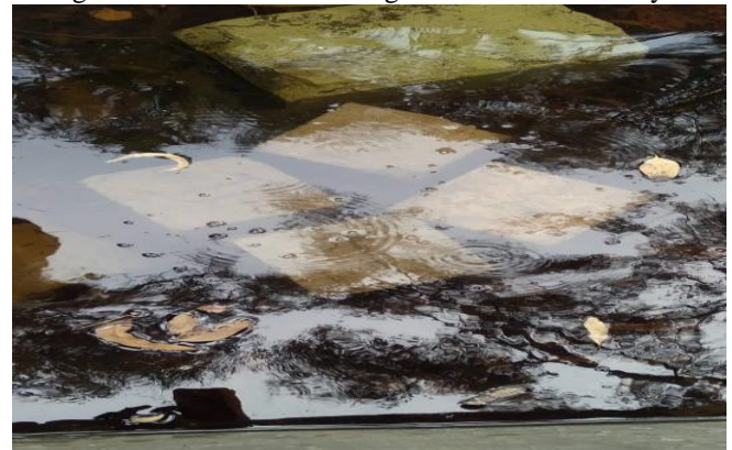
Figure I: Cube specimen kept for curing
