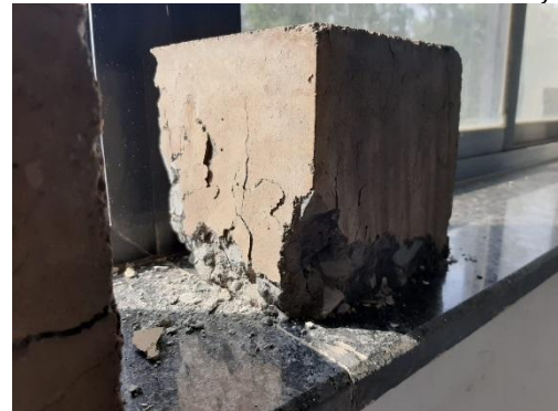
Figure III: Failed concrete specimen
