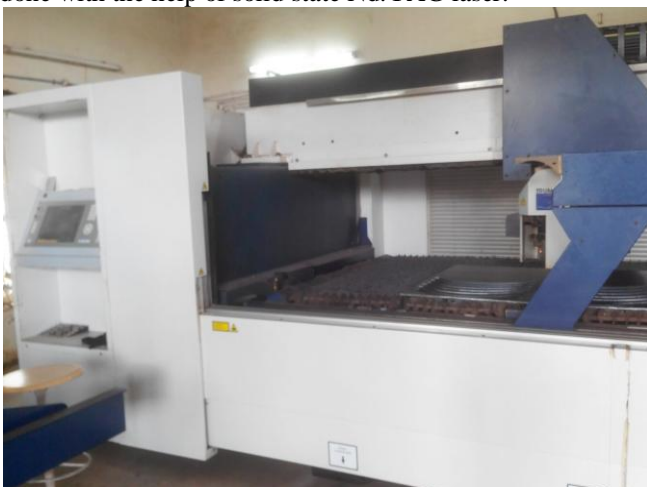
Fig 2.1. Solid state Nd:YAG Laser(Courtesy: Sun India Company)
