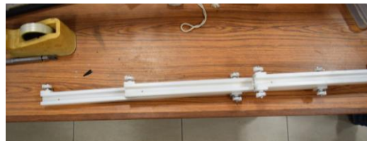
Figure 12 Fabricated linear slide
