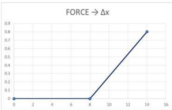
Figure 7 Compression of spring for given force
