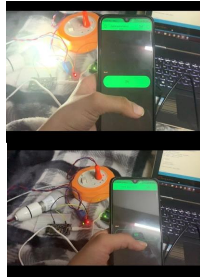
Fig 16: bulb turn on and off by blynk app
