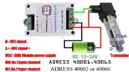
Connection Infrared sensor and modbus converter
